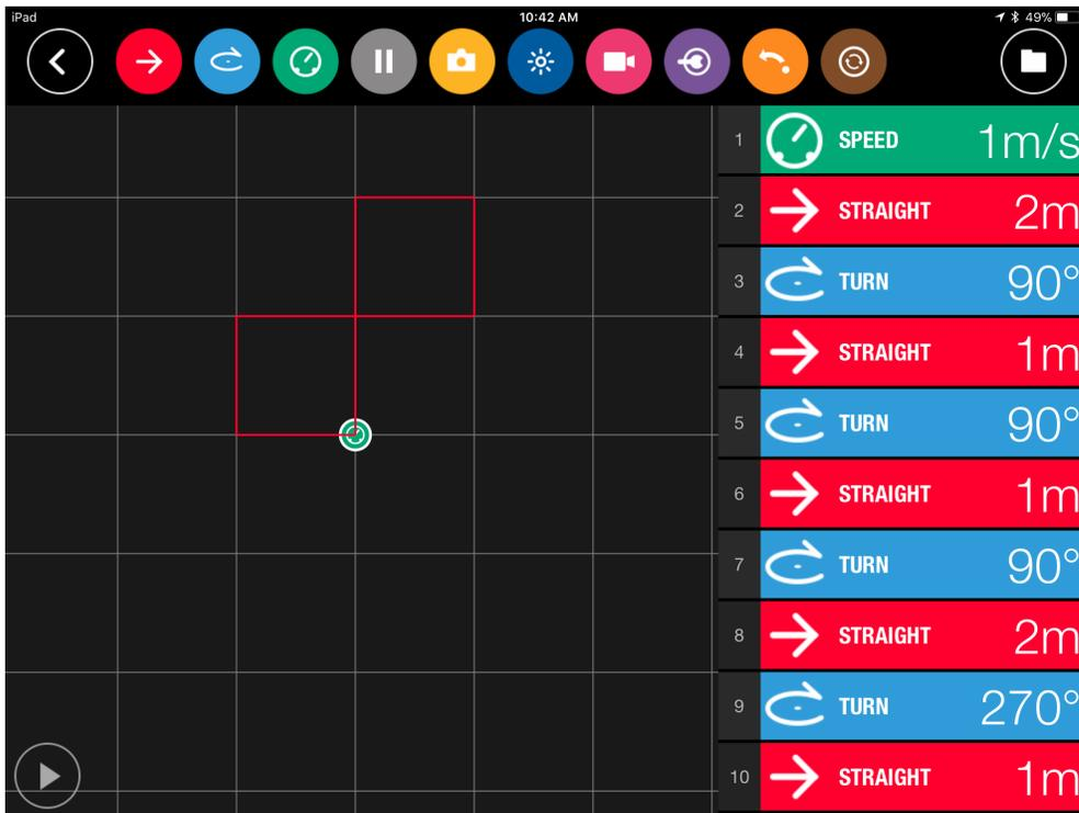
Using the Parrot app, this is the code to direct the drone's motion shown in the movies. Note that commands 11 to 13 to bring the drone back to the starting position are scrolled off the display. Loops are not available. Also, note the command "turn 270" to initiate a left hand turn.
