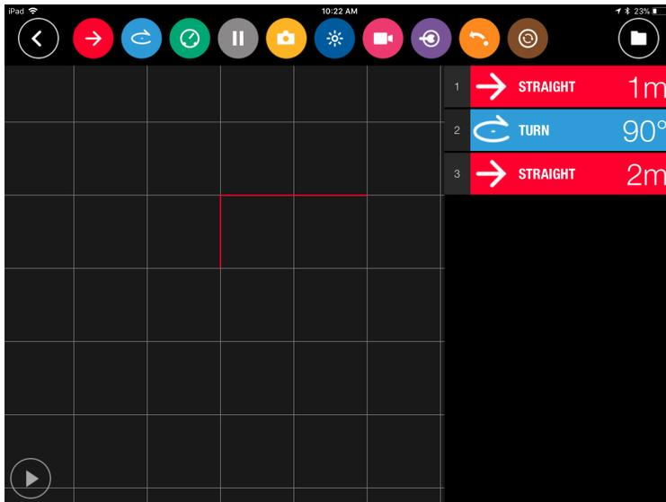
drone motion defined by the code is displayed in red on the grid. This code directs the drone to move forward 1m, turn right, and move forward 2m. The drone motion is very accurate (accepting some slippage due to lack of friction between tires and wood floor) in hitting node points as shown in the above movies.
