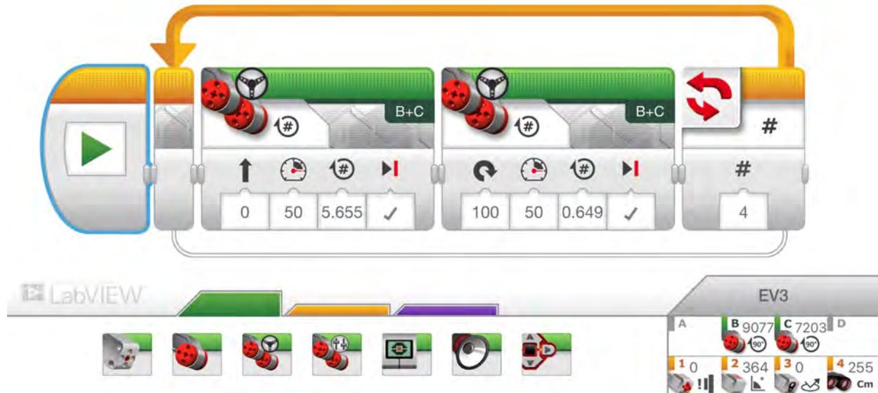
two “move-steering” command blocks. The sensors, which are not currently being used, are connected to ports 1, 2, 3, 4. The code consists of 2 “move-steering” blocks contained within a loop to repeat 4 times. Four input parameters are required and their meaning changes with the mode chosen for the command by clicking the clockwise arrow in the upper left corner of the command. The first move-steering block to direct EV3 to move in a straight line for 1m requires 4 input parameters.
