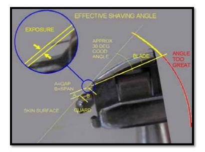
Aggressiveness of a safety razor can be thought of as the degree to which a blade is exposed to the face and beard. Aggressive razors have a large blade gap. A large blade gap leads to quick hair removal, but since more of the blade is exposed to the skin, there is greater risk of nicks and cuts.
