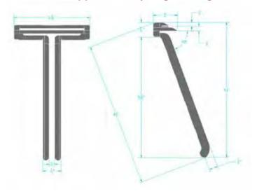
Two things are apparent in the left view. I like the 2 large horizontal gaps which will allow shaving cream and hair to easily pass through and keep the cutting edge clean. However, I'm not sure I like the large width (39 mm) of the shaving head. This will take some time getting used to since it is 11mm longer than my old Schick safety razor. The reason for the large head is to insert Feather Artist Club Razor Blades which are the best on the planet. More about blades later.
