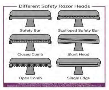
This gets further complicated if you consider safety bar design. The safety bar sits just below the razor blade. This ensures that the blade is properly guarded to avoid accidental cuts and nicks. However, the way these are designed will change the type of shave you experience. Flat edges tend to be gentler when the blade meets the skin while combed guards will be more aggressive.
