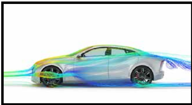
External aerodynamics simulation performed with Altair ultraFluidX on the Altair CX-1 concept design, modeled in Altair Inspire Studio
