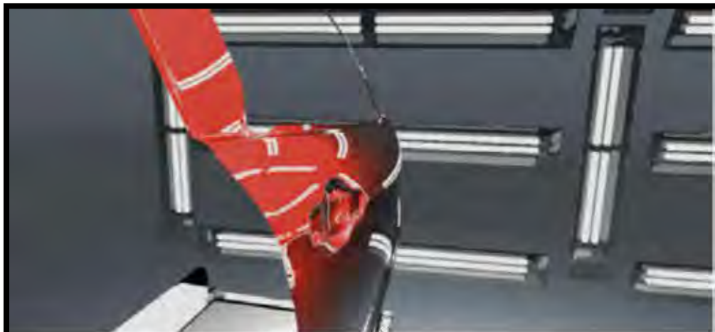
Surface quality analysis in a virtual light room with ESI PAM-STAMP
