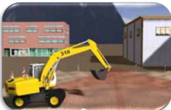
Figure: Excavator model evolving in a bumpy environment used for sensor perception algorithm verification and validation.
