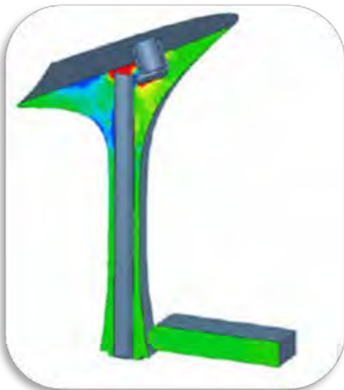
Impact analysis in Marc software. The heel of the shoe is made of an exterior, connection and spine which is impacted by a blunt object. The stress contours are shown with and without the spine.
