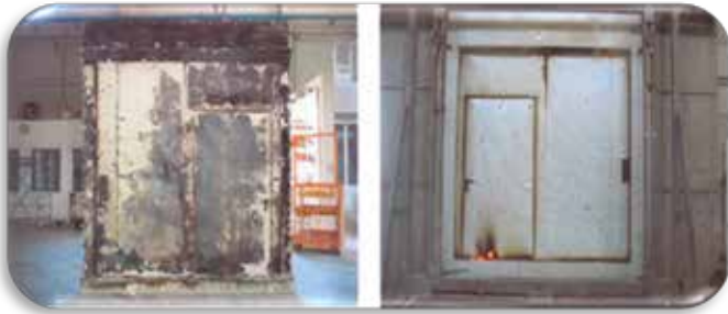
Fig.1: Standard fire test for one specimen barrier including a pass door – Exposed side (left side) and unexposed side (right side) after fire resistance test
