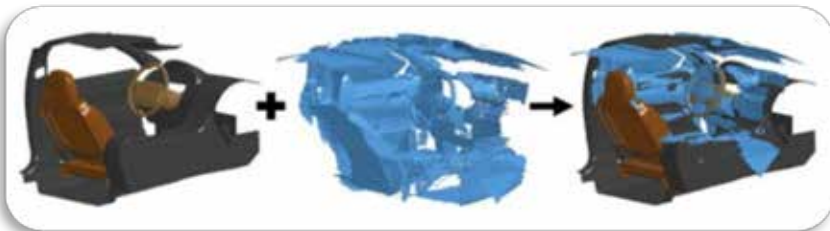
Figure 1. Rigid transformation of the simplified vehicle model to approximate the case vehicle shell geometry.
