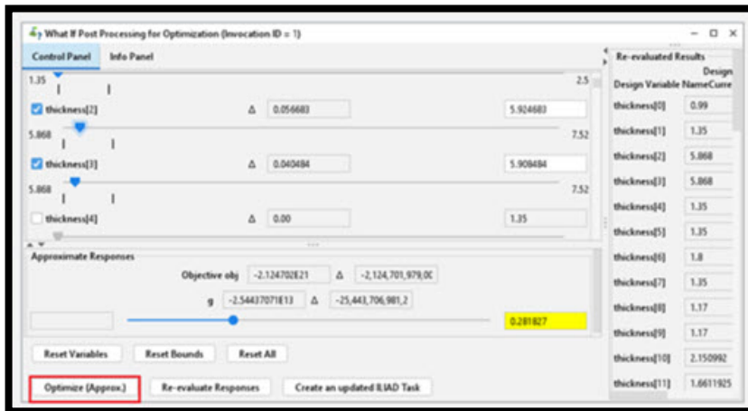
Figure 3: Main What-If panel showing bounds and value of each variable, approximated responses, and reevaluated response values. Approximate optimization highlighted in lower left.
