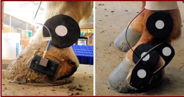
Figure 2. Photograph of hoof extension bar including: (a) A rectangular hoof block which remained rigidly attached to the hoof wall throughout the study period; (b) a hoof wand with kinematic markers to track hoof rotation and translation.
