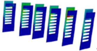
Figure 2: Vertical slices through simulation used in the analysis of environmental uniformity through racking system.
