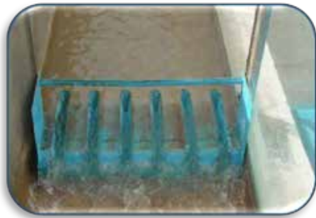
Figure 3 | Channel flow over labyrinth weir with rounded entrance
