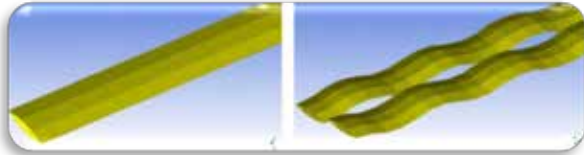
Fig. 5. Finite elements models of the threads of the embroidered structure and the Twaron CT709 fabric.
