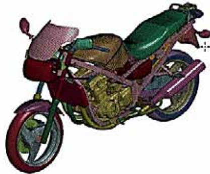
Figure 8. Perspective view of FE motorcycle model without plastic coverings.
