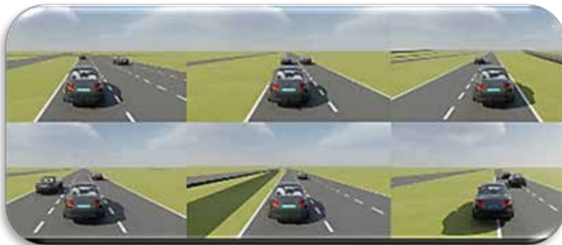
Figure 4: Approach of a stationary vehicle and cut-ins (from right and left), extracted from real-world data, imported in Simcenter Prescan (traffic lights not included in simulation)
