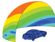
Radiated noise from vehicle at 10 Hz and 140 Hz, by BEM acoustic solver
