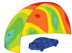
Radiated noise from vehicle at 10 Hz and 140 Hz, by BEM acoustic solver
